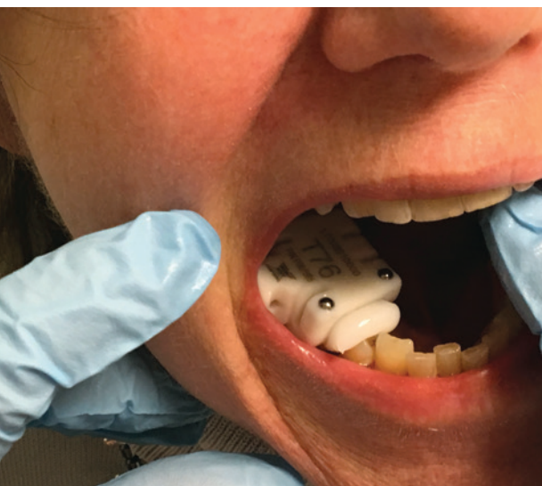
▲ The X-Clip, molded to fit the patient's mouth, has three fiducial markers, or sensors, that track the position of the hand-held instruments relative to the patient's jaw and show it on a computer screen.
