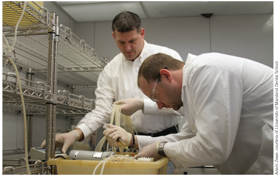
Seeing it through: Mark Shirliff observes bacteria being flushed through to create biofilms on tubing.
